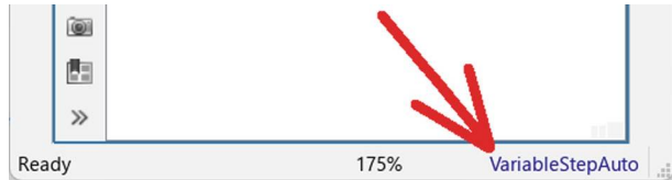
Fig. 12.24 Numerical method used by Simulink to solve the model
